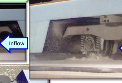
We have validated the results obtained from our snow accretion by comparing them with those obtained from the experiments by the use the snowfall wind tunnel. Additionally, since this snow accretion simulator is made by the distributed memory parallel calculation programing, it allows us to solve a very huge calculation model such as a whole train bogie.
