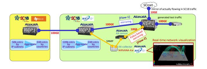
We constructed the 100GE network cooperated with multiple RCP capable nodes and multiple servers. RCP is designed from flexible hardware and can be reconfigured to *Flex Counters*.
